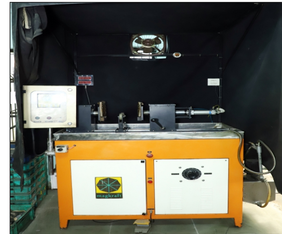
WET TYPE MAGNAFLUX CRACK DETECTION MACHINE (NOS 02)
