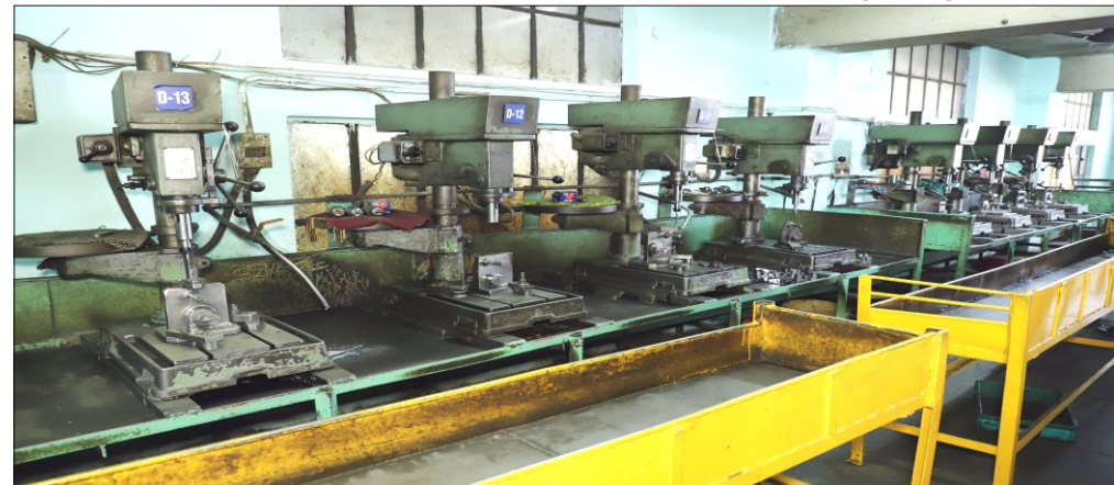
FIFCO MAKE BENCH DRILL DIA 16 MM (22 NOS)
