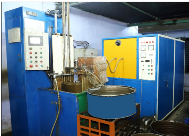
BOSS MAKE PLC CONTROLLED 60 KW INDUCTION HARDENING SETUP (NOS 2)
