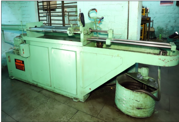
HORIZONTAL HYDRAULIC BROACHING MACHINE 10 T (06 NOS)
