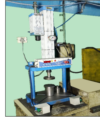
MERCURY PNEUMATIC PRESS 3 T (01 NOS)
